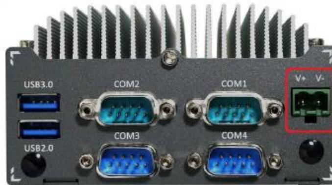
5. Push the terminal block into the power plug until it's firmly attached. Now you can supply the DC power and operate your POC-200.
