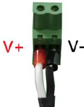
4. Find the 2-pin power plug on the VB-30 which accepts the terminal block. It's located on the right-side of back panel.
