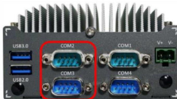
RS485 output is configured on COM1 (indicated below) using PIN 2 (TX+) and PIN 8 (TX-).
